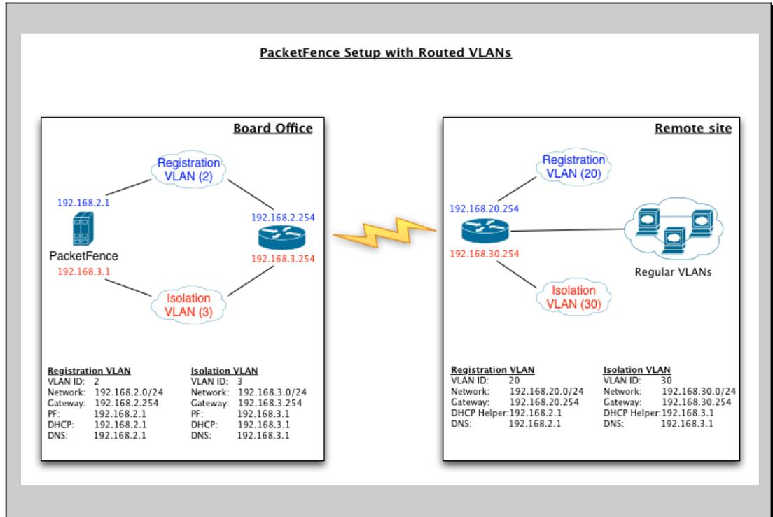
For `dhcpd`, make sure that the clients DHCP requests are correctly forwarded (IP Helpers in the remote routers) to the PacketFence server. Then make sure you followed the instructions in the [DHCP and DNS Server Configuration \(networks.conf\)](#) for your locally accessible network.
