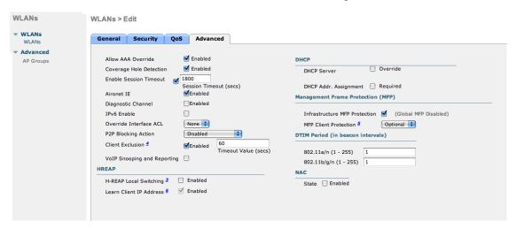
• Edit the non-secure SSID: Enable MAC authentication at level 2
