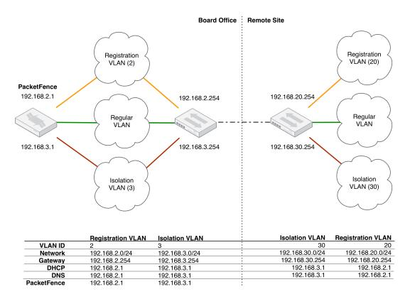
For dhcpd, make sure that the clients DHCP requests are correctly forwarded (IP Helpers in the remote routers) to the PacketFence server.
