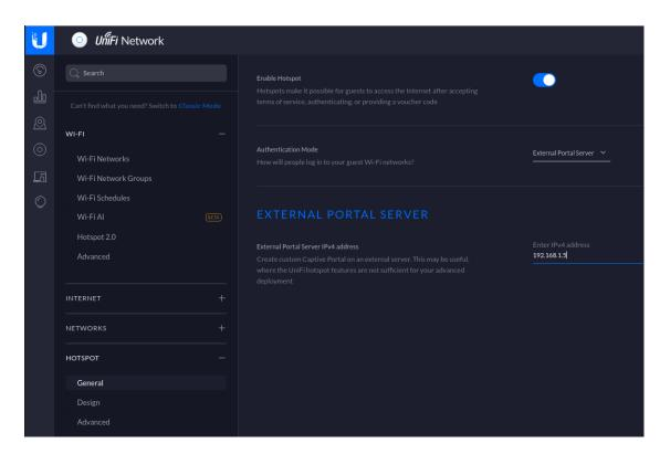
Next, you must allow the device to reach the portal. Go in Settings  $\rightarrow$  hotspot  $\rightarrow$  advanced and configure it as shown below:
